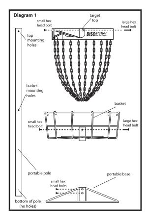
Step 1 BASE - Sit the target base on the ground. Slide BOTTOM of target pole (end with no holes) into base. Insert two 1/4" x 3/8" hex head bolts into threaded holes on base and tighten against the pole.
