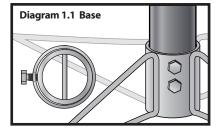
Step 2 BASKET - From the top of the pole slide the basket down and line up the 2 holes for the hex bolt, with the threaded hole on the opposite side of the pole from the third hole in the pole. Insert 5/16" x 2 3/4" hex bolt through basket and pole and tighten nut with wrench. Insert the 1/4" x
