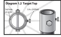
as you put the target top onto the pole. Align target top with the threaded hole on the **opposite** side of the pole from the third hole in the pole. Insert 5/16" x 2 3/4" hex bolt through target top and pole and tighten nut with wrench. Insert the 1/4" x 3/8" hex bolt into the threaded hole on the target top and tighten against the pole.
